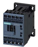
Contactor, AC-1, 18 A/400 V/40  $^\circ\text{C},$  S00, 4-pole, 230 V AC, 50/60 Hz, Spring-type terminal
