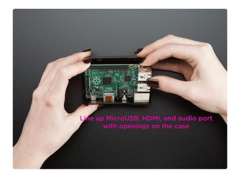
Leave the clear top off, we'll need to access the GPIO header for the PiTFT.
