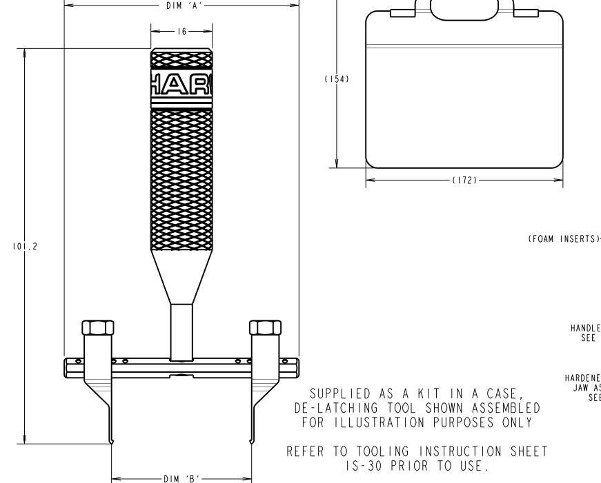
DE-LATCHING TOOL SHOWN ASSEMBLED FOR ILLUSTRATION PURPOSES ONLY REFER TO TOOLING INSTRUCTION SHEET HARDENED ADJUSTABLE-JAW ASSY (2-OFF) SEE NOTE 3 34mm LONG, MULTI-POSITIONAL BAR (I-OFF) 60mm LONG, MULTI-POSITIONAL BAR (I-OFF) DATE APPROVED: MGP CHECKED: S.FLOWER DRAWN:
