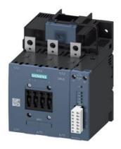
power contactor, AC-3 150 A, 75 kW / 400 V AC (50-60 Hz) / DC operation 96-127 V AC/DC auxiliary contacts 1 NO + 1 NC 3-pole, frame size S6 busbar connections drive: electronic with PLC / SIMOCODE - interface and remaining lifetime signal
