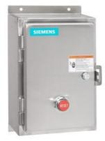
Non-reversing motor starter, Size 3, Three phase full voltage, Solid-state overload relay, OLR amp range 25-100A, Non-combination type, Encl. type 4X 304 S. Steel, Water/dust tight noncorrosive, Standard width enclosure
