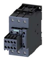
Power contactor, AC-3 80 A, 37 kW / 400 V 2 NO + 2 NC, 230 V AC 50 Hz 3-pole, size S2 screw terminals integrated varistor
