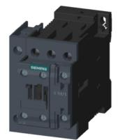
Contactor, AC-1, 50 A/400 V/40  $^\circ\text{C},$  S0, 4-pole, 110 V DC, 1 NO+1 NC, screw terminal
