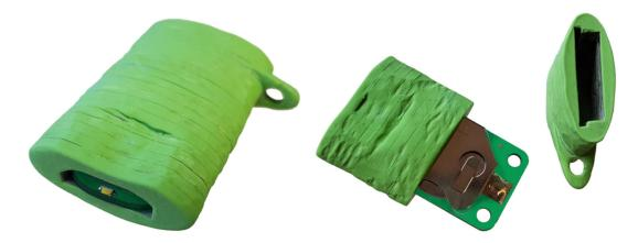
In the second example, the case uses laser cut rubber to create a complete shell around the torch, with a slot at one end to allow the LED light to shine out. The case is made up of segments which are glued together and then slotted over the torch PCB.
