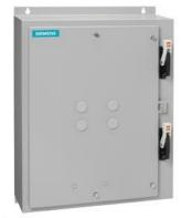
Duplex starter w/o alternator, Size 2, Three phase full voltage, Solid-state overload relay, OLR amp range 13-52A, 190-220/220-240V 50/60Hz coil, Combination type, Two 50A circuit breakers, Encl NEMA type 4X 304 S-Steel, Water/dust tight noncorrosive
