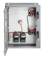
Pump control panel, Duplex controller Starter size 1.75 Solid-state overload relay, OLR amp range 10-40A, 120 VAC coil, Fusible disconnect HOA Sel Sw. and Start P.B., Enclosure NEMA type 3/3R,12 Weather proof outdoor use
