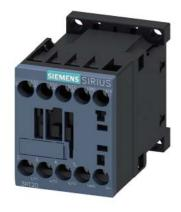
Contactor, 5 HP, 460 / 575 V, 1 NO, 24 V DC, 3-pole, Size S00 screw terminal
