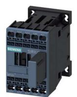
power contactor, AC-3 7 A, 3 kW / 400 V 1 NC, 24 V DC 0.85-1.85\* US, with varistor integrated, 3-pole, size S00, spring-type terminal not expandable with auxiliary switch
