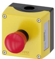
Enclosure for command devices, 22 mm, round, Enclosure material plastic, Enclosure top part yellow, 1 control point plastic, Control point in center, A=EMERGENCY STOP mushroom pushbutton red, 40 mm, rotate-to-unlatch, 1 NC, 1NO, screw terminal, floor mounting, 1xM20 each on top and bottom
