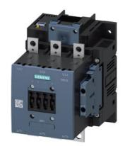
power contactor, AC-3 115 A, 55 kW / 400 V AC (50-60 Hz) / DC operation 21-27 AC/DC, 3 V auxiliary contacts 2 NO + 2 NC 3-pole, frame size S6 busbar connections drive: electronic with PLC interface 24 V DC screw terminal
