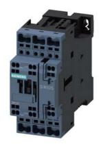
Traction contactor, AC-3 32 A, 15 kW / 400 V 1 NO + 1 NC with solid-state operating mechanism 125 V DC, 0.7-1.25\*Us with integrated varistor 3-pole, size S0 Spring-type terminals
