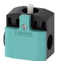
position switch plastic enclosure according to EN 50047, 50 mm device connection 2 x (M20 x 1.5) 1 NO/2 NC slow-action contacts with makebefore-break rounded plunger
