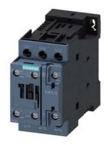
power contactor, AC-3 9 A, 4 kW / 400 V 1 NO + 1 NC, 42 V DC 3-pole, Size S0 screw terminal
