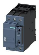
Capacitor contactor, AC-6b 75 kVAr, / 400 V 2 NC, 110 V AC, 50 Hz 3-pole, Size S2 screw terminal
