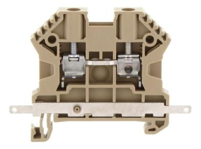
Feed-through terminal, Screw connection, Mounting type: Mounting rail TS 35/7.5, Rated cross-section: 4 mm<sup>2</sup>, Width: 6 mm, Colour: Black
