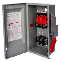
Siemens Low Voltage Circuit Protection Heavy Duty Safety Switches. Type: ENCLOSED, SAFETY SWITCH Std: CSA V. Rating: 240V A. Rating: 60A Wattage: 3W No. Of Poles: 2P F. Rating: 60Hz Action: SINGLE THROW Material: STEEL Enclosure: TYPE 1. 2-3 point mounting holes. O. Cycles: 10000 O. Temperature: (-20F-120F) AMBIENT TEMPERATURE Environmental Conditions: INDOOR
