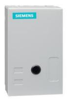
Electrically held lighting contactor, Contactor amp rating 20A, 0 N.C. / 4 N.O. Poles, 110VAC 50HZ/120VAC 60HZ coil, Non-combination type, (no disconnect device), Enclosure NEMA type 1, Indoor general purpose use
