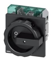
SENTRON, Molded case switch 3LD5 UL, Main switch, 4-pole, certified according to UL489 UL60947-4-1 and IEC60947-3, UL: 30A, SCCR 50kA at 480VAC, Operating power at 480VAC 3-phase: 20hp, IEC: 32A, Operating power at AC-23A at 400V: 15kW, front-mounted, rotary operating mechanism, black, 4-hole mounting of the handle, incl. terminal covers for the infeed side
