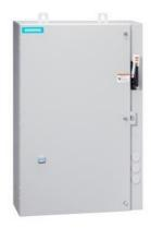
Non-reversing motor starter, Size 1, Three phase full voltage, Solid-state overload relay, OLR amp range 10-40A, Combination type, 60A non-fusible disconnect, Encl NEMA type 4X 304 S-Steel, Water/dust tight noncorrosive, Extra-wide enclosure
