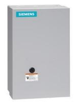
2-speed 3-phase motor starter, Size 1, One winding consequent pole, Constant or variable torque, Solid-state overload relays, Low Spd OLR range 5.5-22A, High Spd OLR range 5.5-22A, 110V 50Hz / 120V 60Hz coil, Enclosure NEMA type 1, Indoor general purpose use
