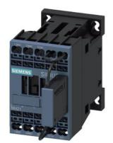
Contactor relay for railway, 2 NO + 1 NC, 110 V DC, 0.7  $\dots$  1.25\* US, with integrated suppressor diode, Size S00, Spring-type terminal suitable for PLC outputs
