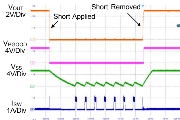
Figure 3. Short Circuit Protection and Recovery
