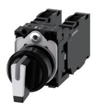
Selector switch, illuminable, 22 mm, round, plastic, white, selector switch, short, 3 switch positions I>O<II, momentary contact type, 10:30h/12h/13:30h, with holder, 2x1NO+1NC, screw terminal
