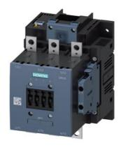
power contactor, AC-3 150 A, 75 kW / 400 V AC (50-60 Hz) / DC operation 200-277 V AC/DC auxiliary contacts 2 NO + 2 NC 3-pole, frame size S6 busbar connections drive: electronic with PLC interface 24 V DC screw
