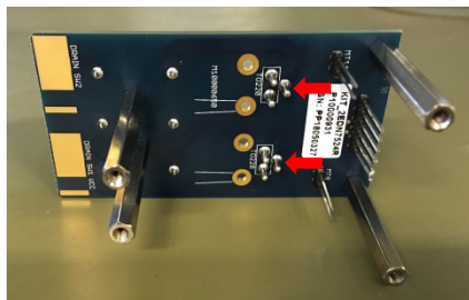
Step 4 TO-220 sockets soldering
