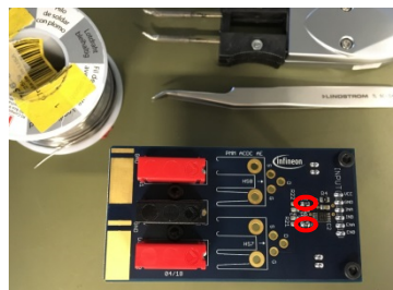
Step 5 MOSFETs placement into the sockets
