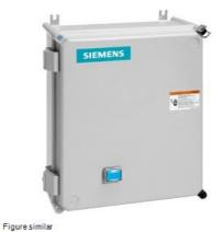
Non-reversing motor starter, Size 2 1/2, Three phase full voltage, Amb. compensate bimetal OLR, Contactor amp rating 60A, 208VAC 60Hz coil, Non-combination type, Enclosure type 4X fiberglass, Water/dust tight noncorrosive
