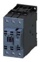
Power contactor, AC-3 65 A, 30 kW / 400 V 1 NO + 1 NC, 20-33 V AC/DC communication-capable, with varistor, 3-pole, Size S2, Spring-type terminals
