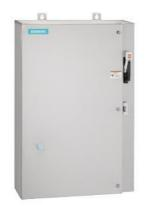
Non-reversing motor starter, Size 2 1/2, Three phase full voltage, Solidstate overload relay, OLR amp range 25-100A, 24VAC 50-60Hz coil, Combination type, 100A fusible disconnect, 100A/600V fuse clip, Encl NEMA type 4X 304 S-Steel, Water/dust tight noncorrosive, Extra-wide enclosure
