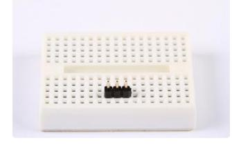
Position the header Trim the header to size if needed and place long-pins-down in the breadboard.
