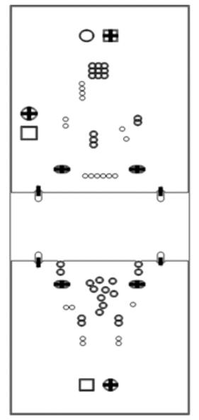
Figure 5. SN6501EVM Ground Plane View
