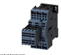
Power contactor, AC-3 38 A, 18.5 kW / 400 V 2 NO + 2 NC, 220 V AC 50/60 Hz, 3-pole Size S0, Spring-type terminals Removable auxiliary switch
