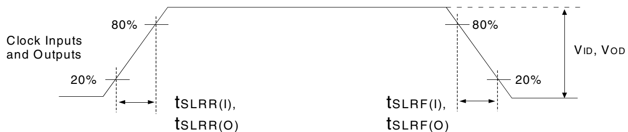
Figure 8. Input and Output Slew Rates
