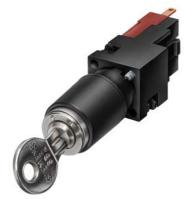
Key-operated switch, 16 mm, round, plastic, CES, 3 switch positions I-O-II, latching, Actuating angle 2 x 62 degree, key removal O, 1 NO, 1 NO
