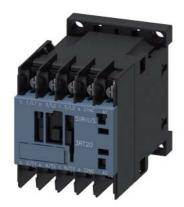
Contactor, AC-3, 7.5 KW / 400 V, 1 NC, 100 V AC, 50 Hz, 100  $\dots$  110 V, 60 Hz, 3-pole, Size S00, Ring cable lug connection
