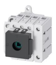
Load disconnector 3LD3, lu 63 A Main switch 3-pole + N Rated operating capacity at AC-23 A at 400V 22.0 kW Installation in distribution boards, Basic switch without Knob-operated mechanism with auxiliary switch 1OE + 1S
