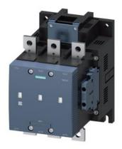
vacuum contactor, AC-3 265 A, 132 kW / 400 V AC (50-60 Hz) / DC operation 200-220 V AC/DC auxiliary contacts 2 NO + 2 NC 3-pole, frame size S10 busbar connections drive: conventional
