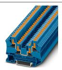
Feed-through terminal block, nom. voltage: 1000 V, nominal current: 41 A, connection method: Push-in connection, Rated cross section: 6 mm², cross section: 0.5 mm² - 10 mm², mounting type: NS 35/7,5, NS 35/15, color: blue
