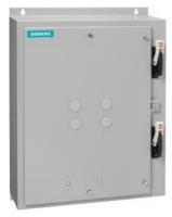
Duplex starter w/ alternator, Size 2, Three phase full voltage, Amb compensate bimetal OLrelay Contactor amp rating 45Amp 110V 50HZ / 120V 60HZ coil, Combination type, Two 60A disconnect switches Enclosure NEMA type 1, Indoor general purpose use
