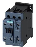
power contactor, AC-3 12 A, 5.5 kW / 400 V 1 NO + 1 NC, 100 V AC, 50 Hz 100-110 V, 60 Hz, 3-pole Size S0, screw terminal
