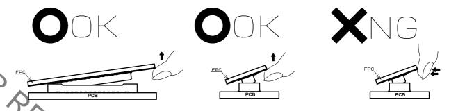
(3) IF THE FPC IS NOT RIGID, THE CONNECTOR CAN BE BROKEN. PLEASE CHECK THE ACTION OF THE FPC TO BE USED REPEATEDLY AT THE TIME OF TRIAL PRODUCTION. BE CAREFUL TO UN-MATE THEM FROM THE PITCH DIRECTION. PULLING IT FROM THE CORNER CAN ALSO RISK TO PUTTING STRESS ON CONTACTS.
