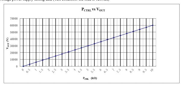
Figure 4. P<sub>CTRL</sub> vs. V<sub>OUT</sub>
