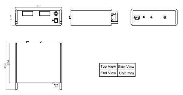
Figure 7. Dimensions for AHVAC60KVR5MABT
