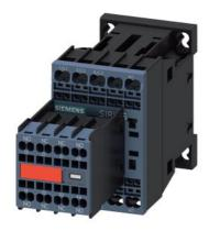
Power contactor, AC-3 12 A,  $5.5~\rm kW$  /  $400~\rm V$  2 NO + 2 NC,  $110~\rm V$  AC,  $50~\rm Hz$  120 V,  $60~\rm Hz$  3-pole, Size S00 Spring type terminal Captive auxiliary switch
