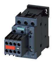
Power contactor, AC-3 32 A, 15 kW / 400 V 2 NO + 2 NC, 230 V AC 50/60 Hz, with inserted varistor 3-pole, Size S0 Screw terminal Captive auxiliary switch
