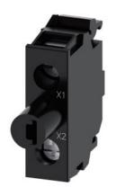
LED module with integrated LED 24-240 V AC/DC, amber, screw terminal, for floor mounting, Z=50-unit packaging
