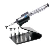
V8901-KIT-B PEN-VAC™ with five bent probes mounted with cup sizes 1/8" (3.18mm), 3/16" (4.76mm), 1/4" (6.35mm), 3/8" (9.53mm), 1/2" (12.7mm) diameter. Three straight probes mounted with cup sizes 1/4" (6.35mm), 3/8" (9.53mm), 1/2" (12.7mm) diameter. Includes Vacuum Pen holder with eight locations for holding your probes and cups.
