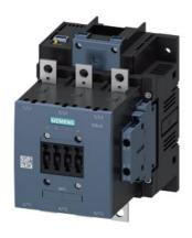
Traction contactor, AC-1 275 A, 690 V Coil 24 V DC x (0.7-1.25) PLC input 24-110 V DC Auxiliary contacts 2 NO + 2 NC 3-pole size S6 Busbar connections Coil connection: screw terminal
